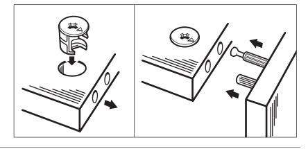
Using the #2 Phillips screwdriver, rotate the Cam Devices a half turn clockwise until snug.
