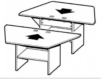
**2.** Align the tops together. Adjust the Levelers (H5) to level both Workstations at the same height.
