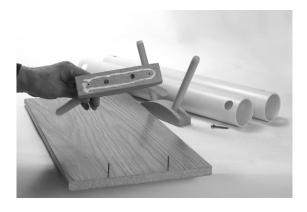
**STEP 1** - Apply an oval-shaped bead of glue (Elmer's or other white glue) to the bottom of one doweled bracket.
